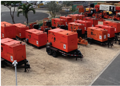
Dri-Prime Pumps for Sewer Bypassing & Dewatering
